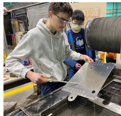
On this page: Learning about pneumatics (top left); working on the swerve drive base (top right); and cutting custom parts using water-jet technology (above)
